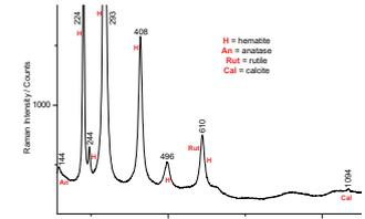
Figure 16.- Raman spectrum collected on a brown zone
