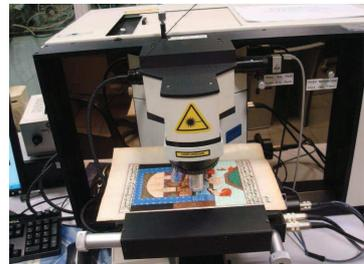
Figure 1.- Experimental set-up of the micro-Raman system employed for manuscript analysis. Materials Science Institute of Seville.
