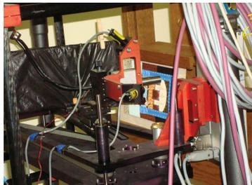
Figure 2.- Experimental set-up of the XRD/XRF portable system employed for manuscript analysis. Centre de Recherche et de Restauration des Musées de France.
