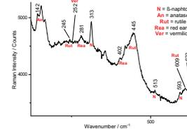
Figure 13.- Raman spectrum on a red zone
