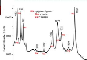
Figure 19.- Raman spectrum collected on a green zone
