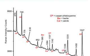
Figure 20.- Raman spectrum collected on a blue zone
