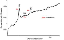
Figure 11.- Raman spectrum collected on the red letter
