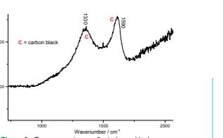
Figure 9.- Raman spectrum collected on a black area
